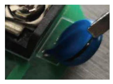
The electronic original has been damaged by the overload protection after the working voltage exceeds the specified voltage.
