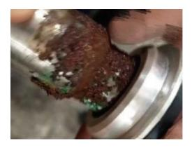
As the solenoid valve is opened for a long time, the damp dust in the pipe has rusted and accumulated on the iron core, causing the solenoid valve to not close properly.
